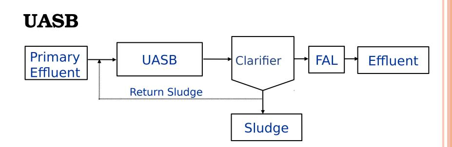
Capital cost : Rs. 2.5 - 3.6 million per MLD O & M Costs : Rs. 0.08 - 0.17 million/year/MLD installed capacity Land Requirement :0.2 - 0.3 hectares/MLD installed Capacity Energy Requirement : 10 - 15 KWh/ML treated
